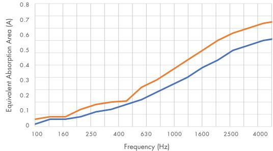
All results are reported in Metric Sabin - per unit. Equivalent sound absorption area according to ISO 354 Measurement of sound absorption in a reverberation room. Average Absorption (Sabins per unit) calculated at one-third octave bands centred on 250 Hz, 500 Hz, 1000 Hz and 2000 Hz. and rounded to the nearest 0.05.
